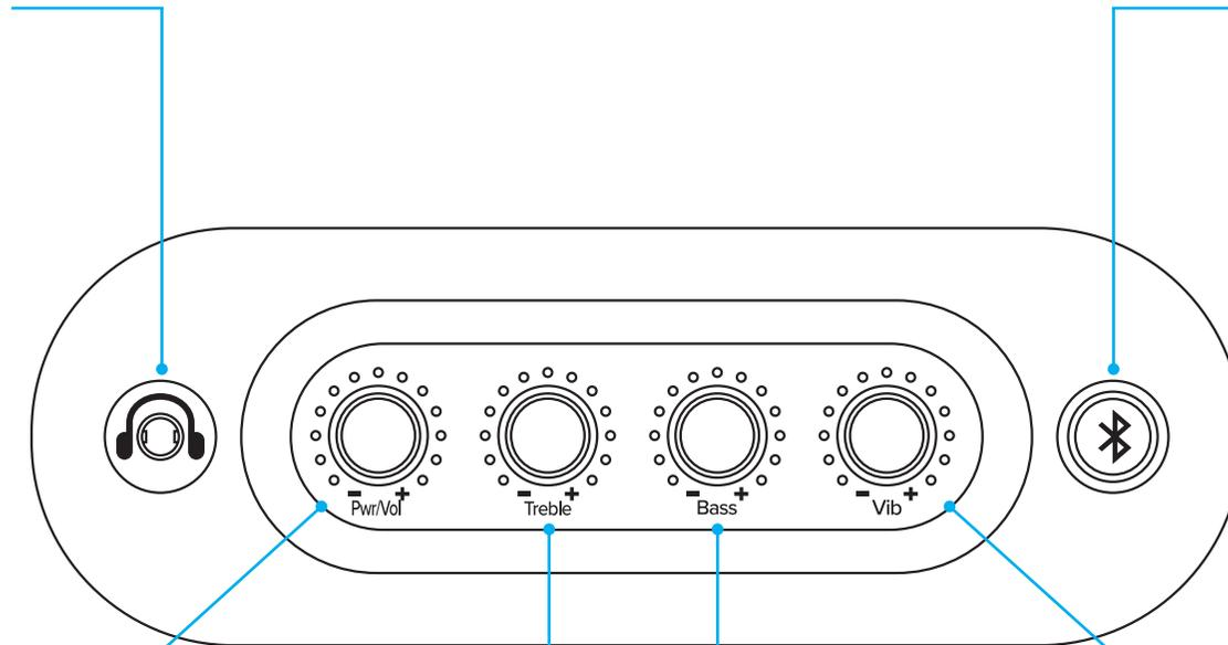
The **Bluetooth button** is used to turn Bluetooth audio function on, and to setup connection between seats.
